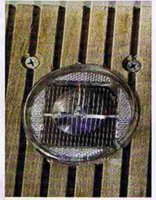
Leaves, sand or dirt can cover up one or more solar cell segments. This results in a total output which is too low to charge the battery. The same will happen on a cloudy day when there is too little light to charge the battery, which will consequently be empty after a few days.
